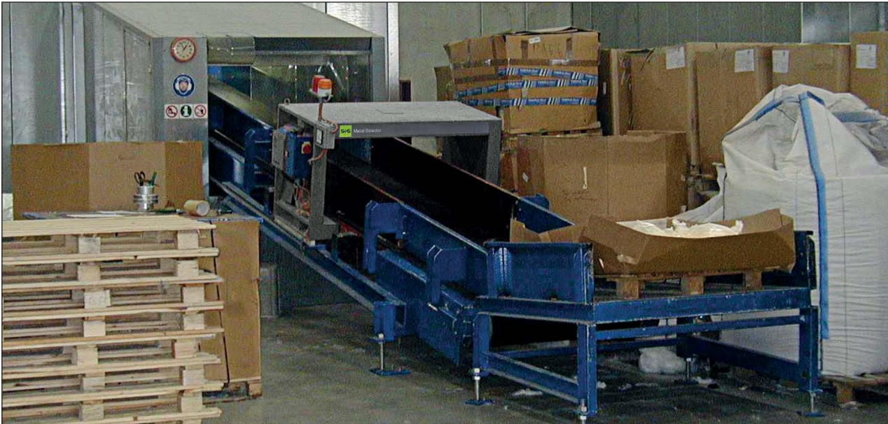
Tunnel metal detector DLS analysing recycling material before the granulator.
